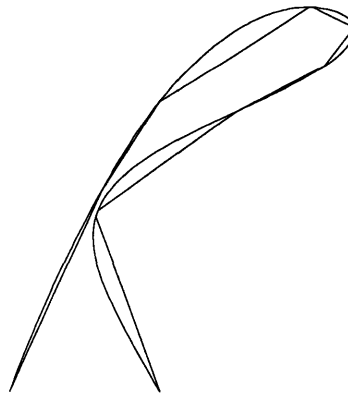
Figure 3-17: A composite curve with constriction and its approximation guaranteeing a prescribed tolerance and the existence of a homeomorphism between the exact and approximating curves
