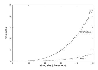
Figure 9: Solving time as a function of string size, on contextfree-grammar intersection constraints. Results are averaged over 100 randomly-selected pairs of context-free grammars. Section 5.4 describes the experiment.
