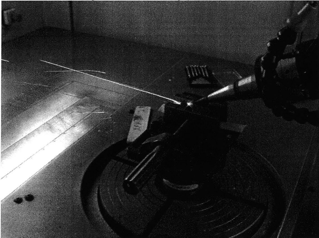
Figure 11 – Laser Drilling of a Test Piece
