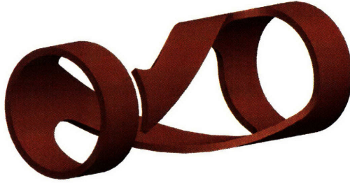
Figure 1-3: Right hand polarized half-helical antenna (RH-HH), used to excite predominantly the m = +1 mode; the helical arms twist counterclockwise away from their originating ring rotating 180^\circ before terminating on the second ring, setting the antenna length at one half the axial wavelength.
