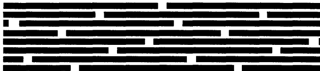
Figure 2.6: Diagram of a bundle of discontinuous CNTs where the length of individual CNTs is less than the length of the overall bundle [65].
