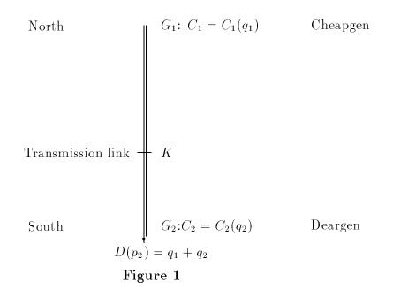
Finally, there is a transmission line linking the North with the South which has a fixed capacity equal to K. The nondepreciated capital and operating costs of this link are assumed to be recovered separately from consumers in lump sum charges net of revenues produced by
