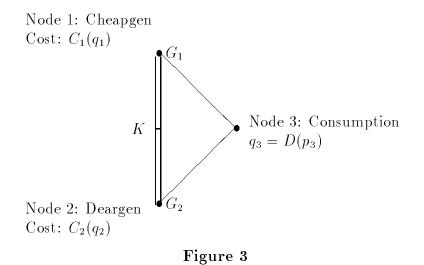
and assume that the three links have equal length and impedance. We focus on the case in which the transmission line between the two generation nodes is congested, which is the direct analog of the two-node network and then discuss briefly how the analysis changes for different patterns of congestion.
