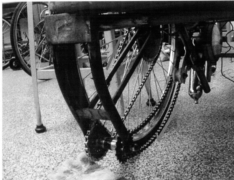
Figure 8: Two-stage gear reduction. This figure shows the relative placement of the gear reduction in respect to the motor. The arrows show the relative motions of the chains.
