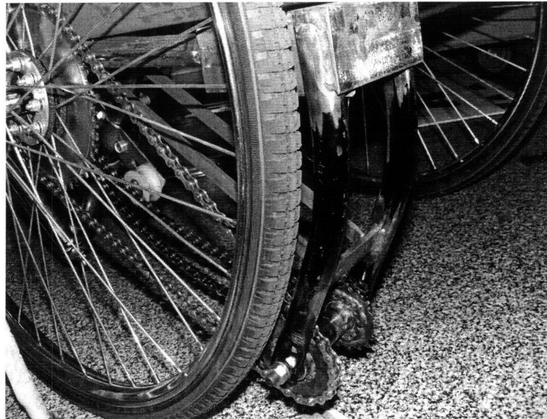
Figure 9: Two-stage gear reduction- external view. The reduction lies very close to the rear wheel in order to minimize the chain length and avoid derailing.
