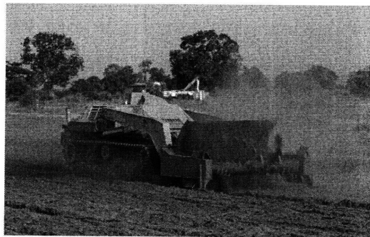
Figure 6: Landmine Removal Using Flail Photo courtesy of US Department of Defense
