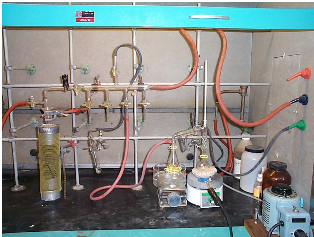
Figure 1. Vacuum distillation apparatus for pyruvic acid. See your TAs for details.
