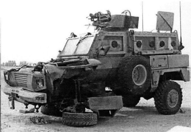
Figure 1-2: BAE's RG-31 damaged by an IED attack obtained from [7]
