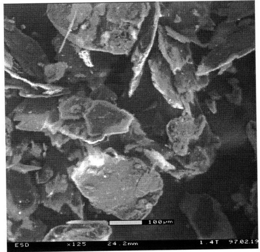
Figure 3-5B. SEM of Graphite Powder, x125(2)
