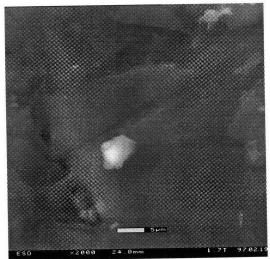
Figure 3-5D. SEM of Graphite Powder, x2000
