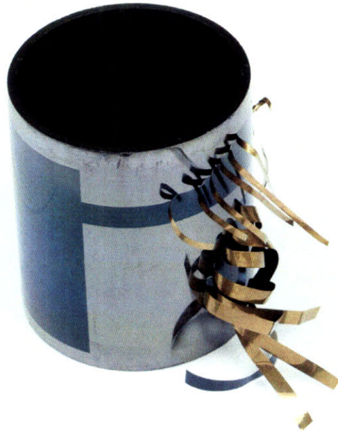
Figure 3-12: Gold backed polypyrrole ribbon actuators partially removed from a glassy carbon crucible.
