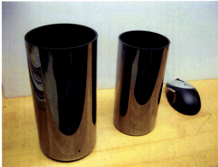
Figure 3-14: Larger crucibles that enable the creation of longer conducting polymer ribbons.
