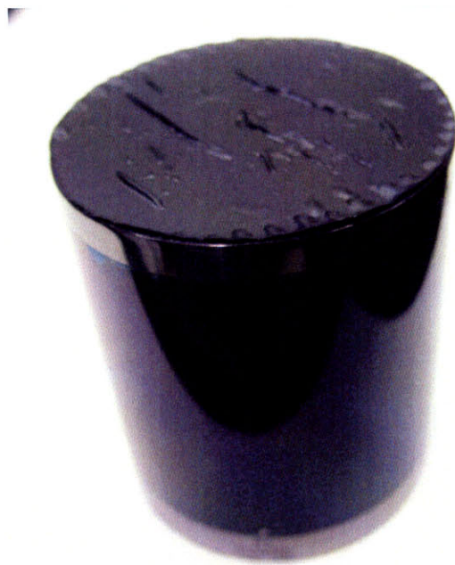
Figure 3-3: A polypyrrole film that has been electrodeposited onto a glassy carbon crucible. The top end surface of this crucible is masked with a black tape. The upper and lower edges of the crucible were masked with a polyimide tape during deposition and removed before this photo was taken, thus revealing the difference between the shiny crucible finish and the matte polypyrrole film.
