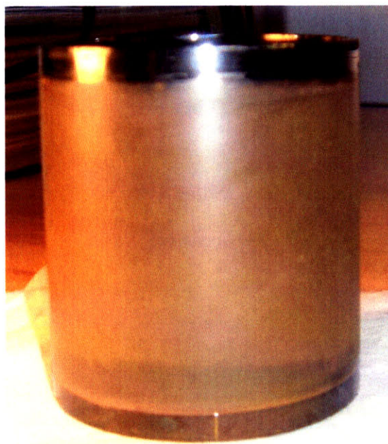
Figure 3-11: Glassy carbon crucible that has been electroplated with gold prior to being electrodeposited with polypyrrole.
