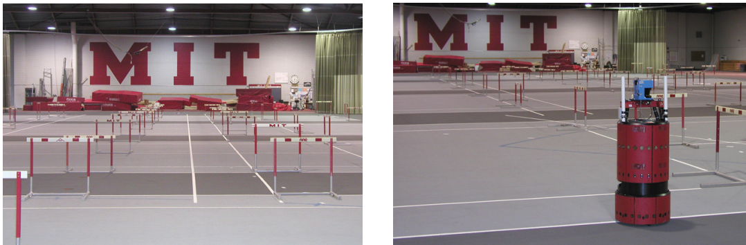
Figure A-1: The experimental setup for the hurdles dataset. The environment consists of 64 track hurdles positioned on the baselines of four adjacent tennis courts. The iRobot B21r robot is equipped with a laser scanner mounted near the base of the vehicle that provides measurements of range and bearing to the hurdle legs within its field-of-view. Note that the second laser scanner affixed at the top of the robot was not used during this experiment.
