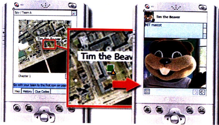
Figure 1.4 Interacting with virtual game objects. Virtual game objects are visible and accessible only through the handheld screen. A player can “visit” a game object by walking into the object’s hotspot.
