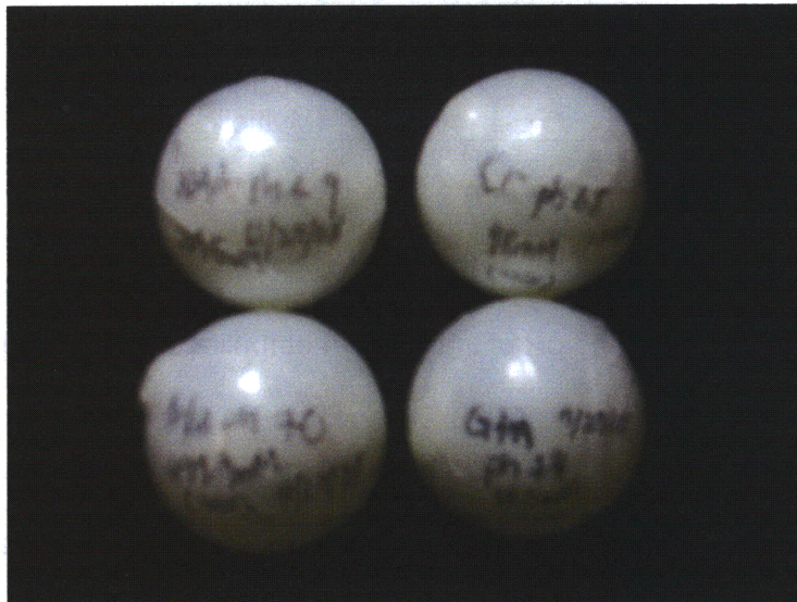
Figure 36. Concentrated solutions of Cr, NAA, Glu and Gln at 98mM, 251mM, 500mM and 180mM respectively were injected into different ping-pong balls of diameter 40mm. The opening was sealed with wax before wrapping the phantom with Parafilm
