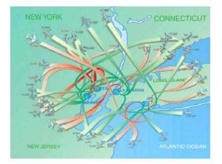
Figure 101: Approach and departure paths for the New York multi-airport system [Source: New York airspace redesign project (FAA, 2006)]
