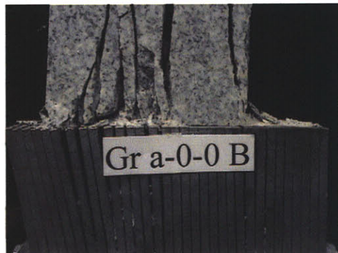
Figure 3.10 – Increased loads for granite specimens caused buckling of the teeth in the brush platens. Many of the teeth in the left third of the platen shown have buckled.
