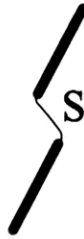
Figure 6.1 – Coalescence pattern observed for the specimen tested with pressure plates but no water pressure inside the flaws. Coalescence is category four (direct shear coalescence).
