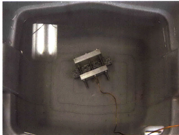
Figure 5.7 – Pressure plates were assembled around the specimen underwater to ensure no air was present inside the control volume. The copper pipe is connected to the PVC.
