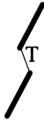
Figure 6.2 – Coalescence pattern observed for the specimen tested with 400 psi flaw pressure. Coalescence is direct (category six).
