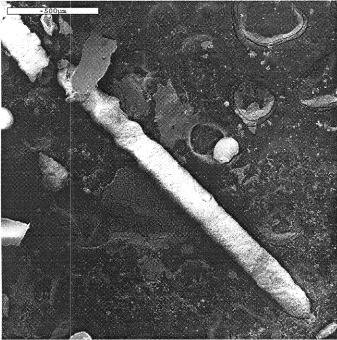
Figure 5.99: SEM of a Line Segment (100 \mu\text{m} spacing, 1 Hz, 2 passes/line, bottom)
