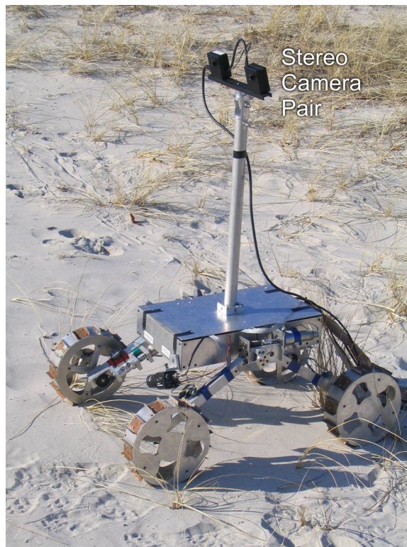
Figure 5-6. TORTOISE, showing location of stereo camera pair
