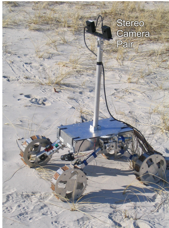
Figure 3-2. TORTOISE, showing location of stereo camera pair
