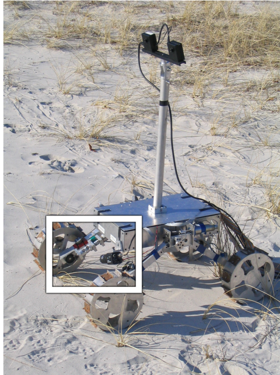
Figure 4-10. Photo of TORTOISE, showing location of local sensor suite
