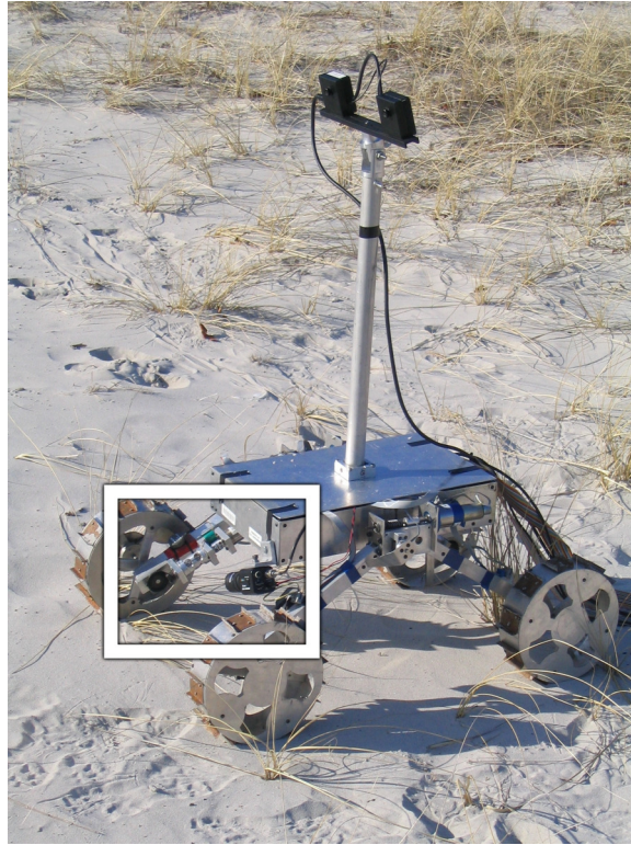
Figure 2-1. Photo of TORTOISE, showing location of local sensor suite
