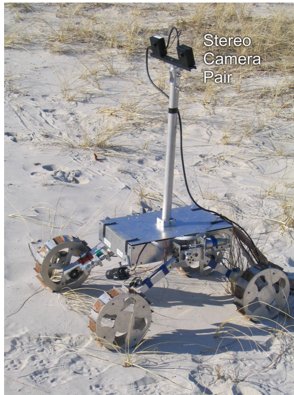
Figure A-1. Photo of TORTOISE, showing location of stereo camera pair
