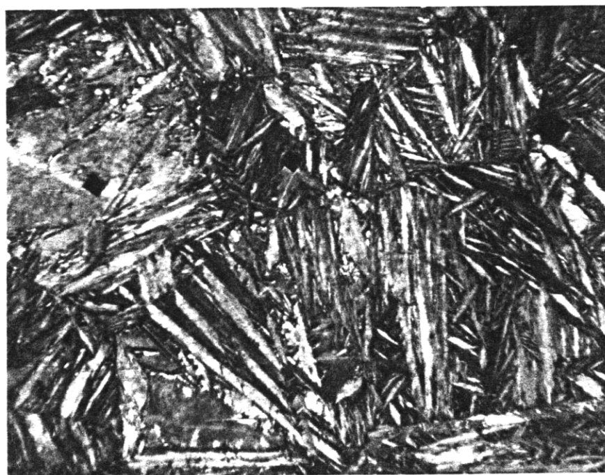
Figure 3-5 Optical micrographs of (a) homogenized S3, (b) S3 aged at 973 K for 3 h.
