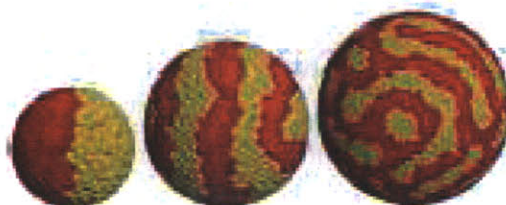
Figure 2.2.3: Simulation generated images of Janus-type ( Left ), ripple domain ( Middle ) and worm-like domain ( Right ) nanoparticles. The figure has been taken from reference 34 without permission.
