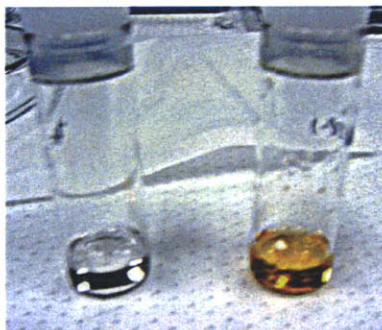
Figure 3.9.7: Picture of the color-change induced in an NBA / ECA mixture with the addition of borate solution.
