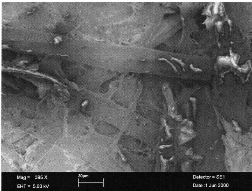
Figure 2-5: Triplex mechanical layer at intermediate magnification.
