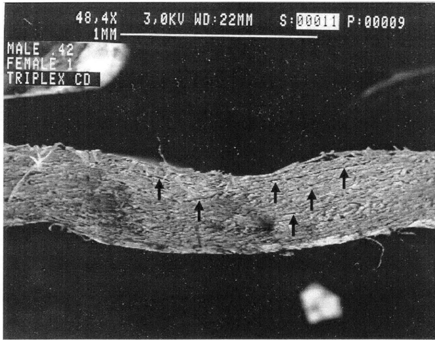
Figure 3-5: Triplex CD bending process at no load (Step 1). Arrows designate damage created by punching process.
