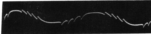
Figure 13. Characteristic waveform of multipath interference in frequency modulation. Modulation frequency = 200 cycles. Frequency deviation = \pm 3000 cycles. De-emphasis time constant = 100 \mu sec. Time delay = 625 \mu sec.
