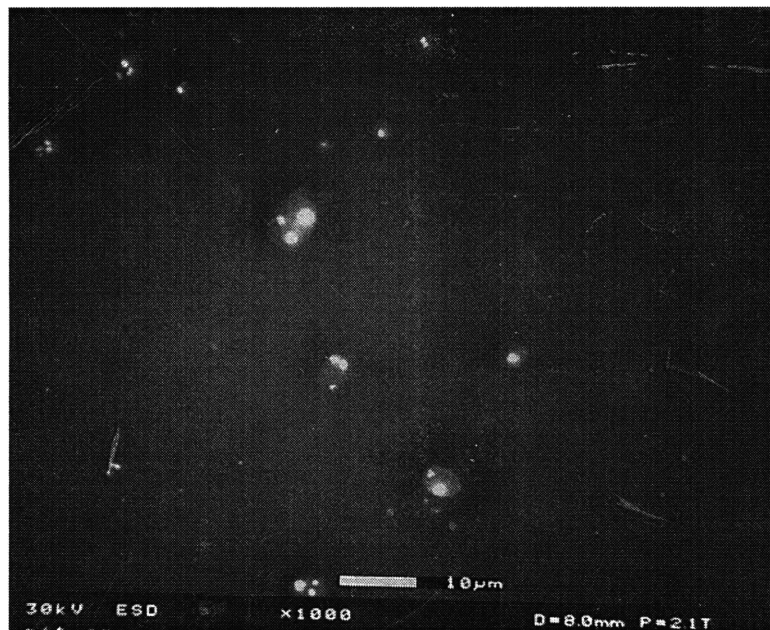
Figure 4-12: Scanning Electron Micrographs of Teflon particles on silicon. Normal load: 2 N. Magnification: 1000.
