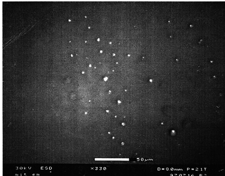
Figure 4-11: Scanning Electron Micrographs of Teflon particles on silicon. Normal load: 2 N. Magnification: 330.
