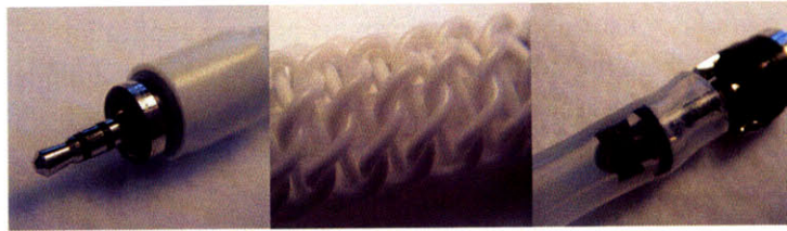
Fig. 8-8 A Senspectra Joint a) radial connector b) eight conductors woven into a diamond braid c) phototransistor embedded in silicon tubing
