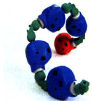
Fig. 5-18 Actives connected with tetrahedrons and programmed with a queen create a spring-like helix
