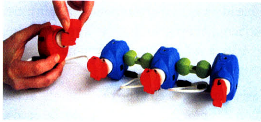
Fig. 5-17 Programming with a queen: all the Actives synchronously copy the motion of the Queen
