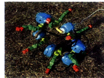
Fig. 5-16 A Topobo “wheel” which rolls like a tank tread
