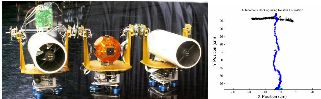
Figure 5. SWARM Phase 1 set-up. SPHERES satellite in center with two telescope sub-apertures (left) and Relative position of SPHERES satellite center (with respect to docking port of sub-aperture) during a successful docking sequence.
