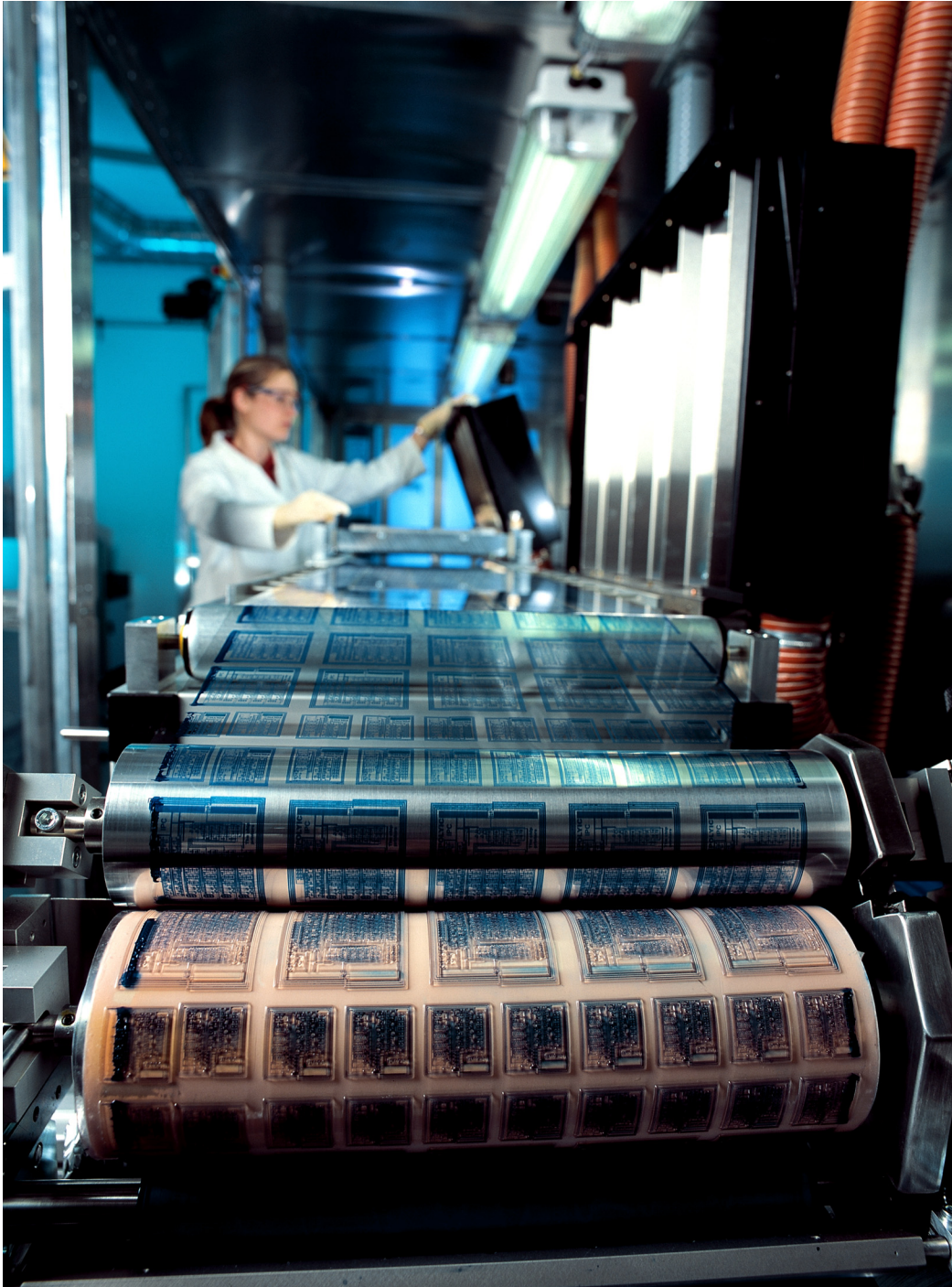
Figure 2-8: Using a laboratory printing machine, printed electronics, such as RFID tags, are being developed by PolyIC. By using a roll-to-roll flexography printing process it is possible to produce large volumes at very low cost. Source: PolyIC press picture
