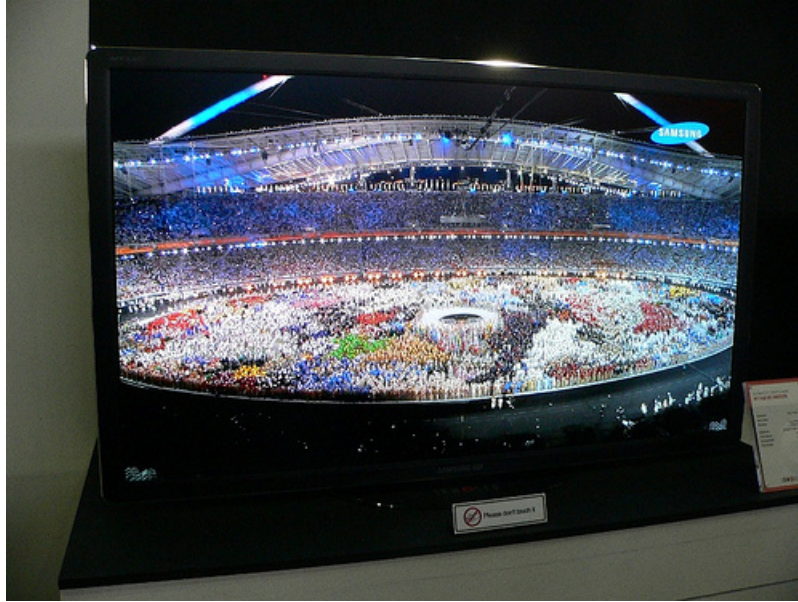
Figure 2-14: Prototype 40" OLED display (worlds largest). Source: Samsung
