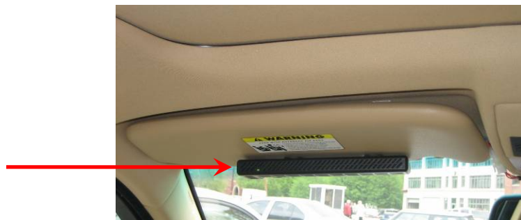
Figure 3: Array microphone used to detect user's voice
