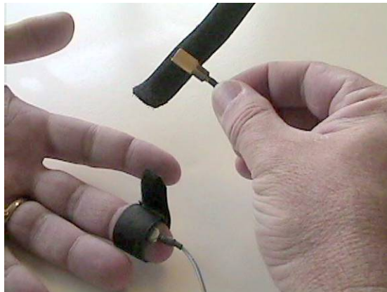
Figure 7: Placement of skin conductance sensors
