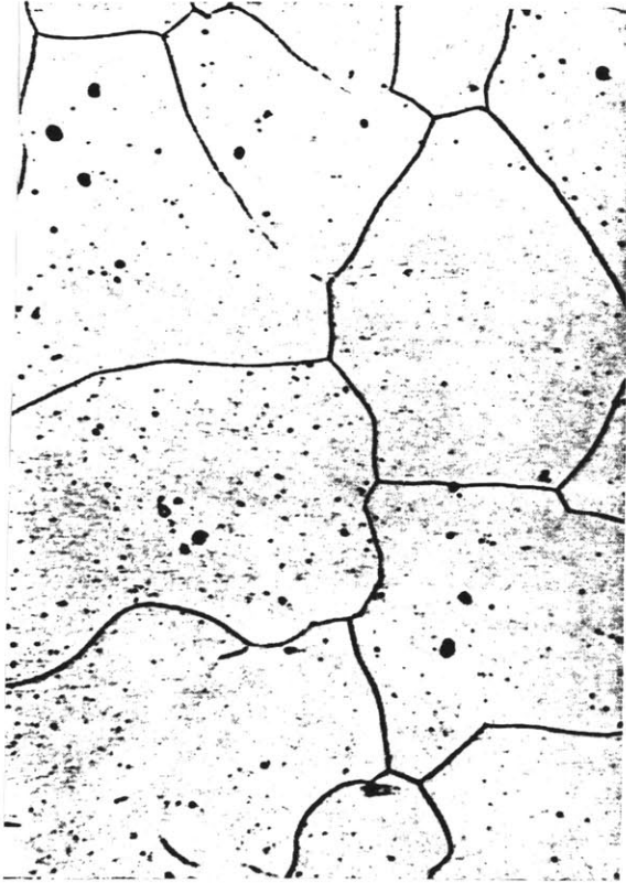
Fig. 19 - Microstructure of untransformed iron. 192X (ref. 32)
