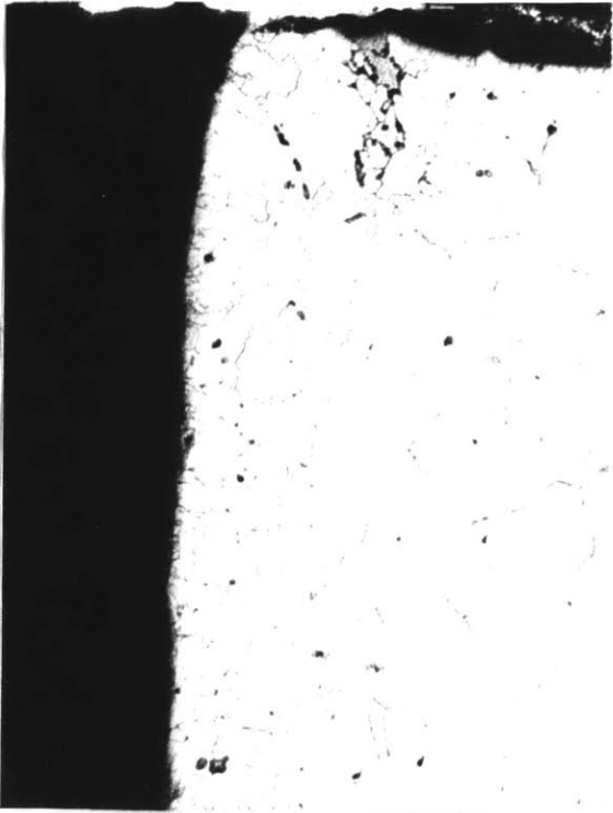
Fig. 28 - Microstructure of rod shown in figure 27 at the electrode junction. 100X
