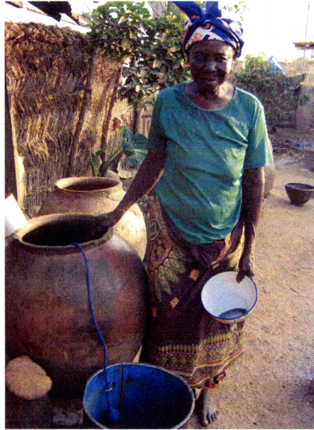
Figure 4.30 Woman with large ceramic pot used as upper container for siphon filter
