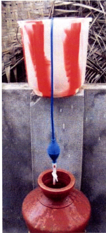
Figure 2.6 Tube, bulb and tap of siphon filter (van der Ven-TWF, 2008)
