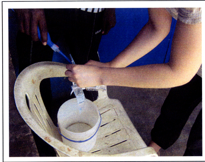
Figure 3.1 Collecting a sample from siphon filter tap into Whirl-Pak bag
