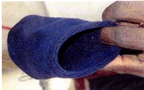
Figure 2.5 Cloth pre-filter (van der Ven-TWF, 2008)
