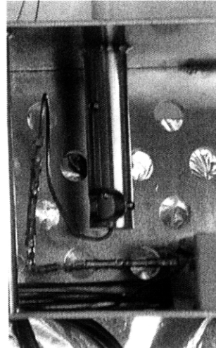
Figure 3-10: Detail of the probe holder and terminal block highlighting the resistor and connection pins/sockets.
