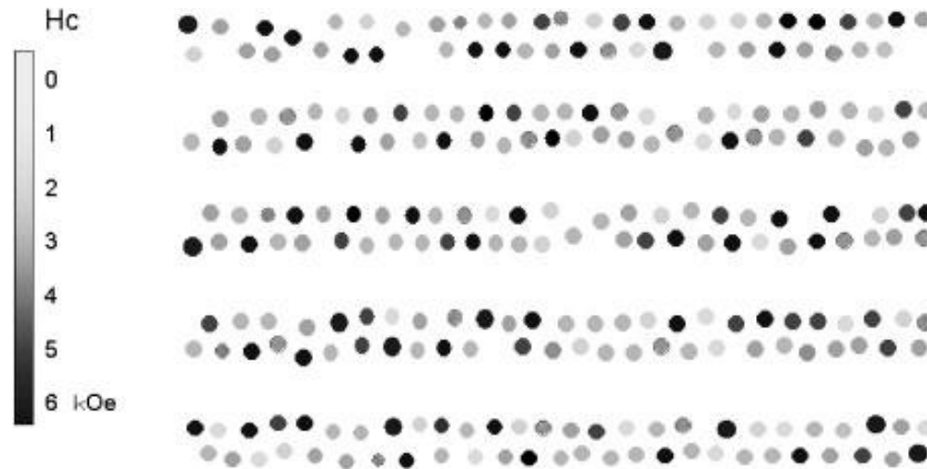
Fig. 2.9. Coercivity distribution map of patterned media obtained by dot-by-dot analysis. The contrast indicates H_c [23].
