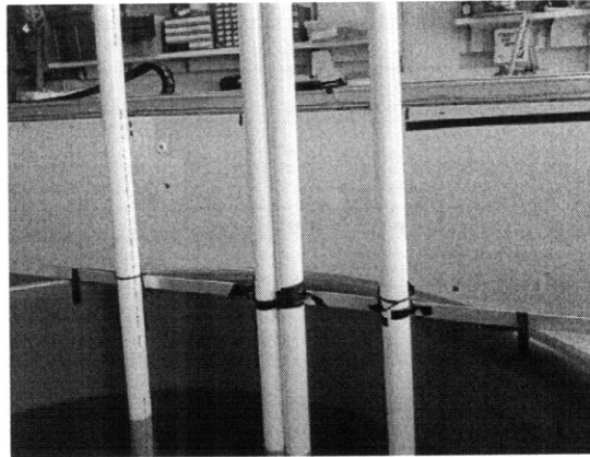
Figure 2-2. Poles strapped on in the tub. The poles are orientated so that the middle poles are closer to one side than other to help with localization.
