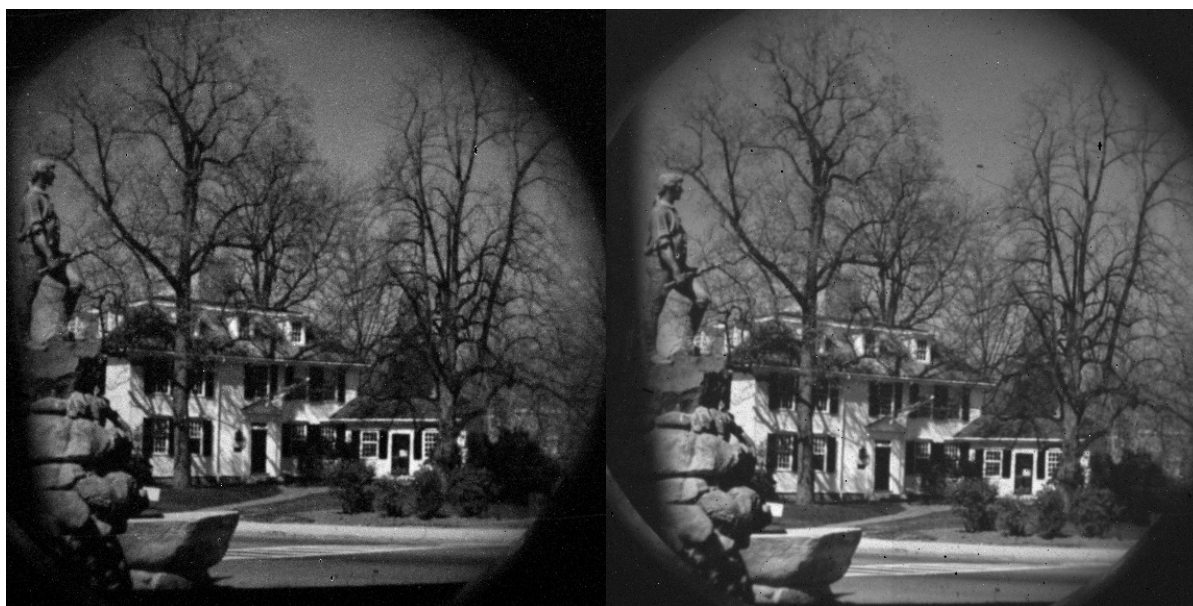
(a) non-dithered conditions, 15 second integration (b) dithered conditions, 60 second integration Figure 9. Images taken with the MBE-processed BI imager operated at +20°C, using conditions shown.
