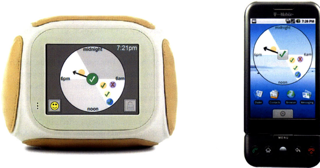
Figure 6: Daily medication clock with quick adherence reporting button shown. When the hour hand enters an adherence interval, the quick adherence reporting button appears, allowing the user to report that all of the medications in that interval were taken. Both devices also use additional awareness prompts such as auditory and vibro-tactile.
