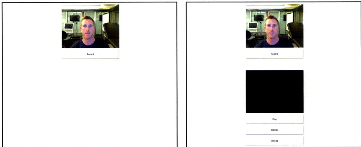
Figure 21: Interface for Recording and Uploading Video Messages. The image to the left shows the initial state of the interface. The user clicks the “Record” toggle button to start recording and clicks it again to stop recording. The image to the right show the interface after a video has been recorded. There is a viewing window and the option to play, delete, or upload the recorded video.
