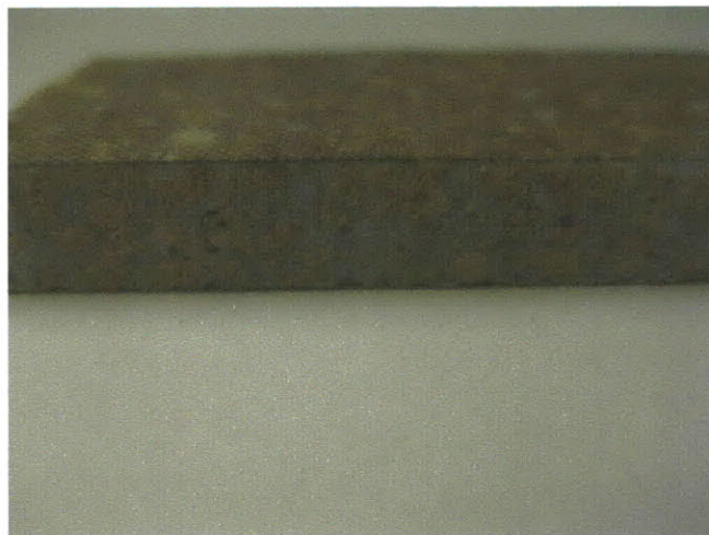
Figure 2.19 A cork composite with resin at 1:2 ratio of cork to epoxy by volume
