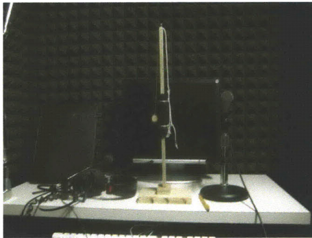
Figure 2.70 The apparatus for sound attenuation test in the booth
