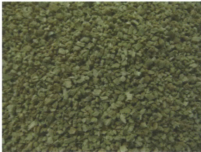
Figure 2.15 The medium size of cork granules: 2-3mm
