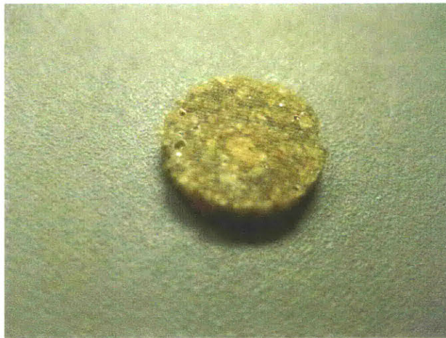
Figure 2.81 A cork specimen for thermal conductivity test
