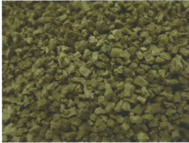
Figure 2.14 The biggest cork granules: 4-5mm
