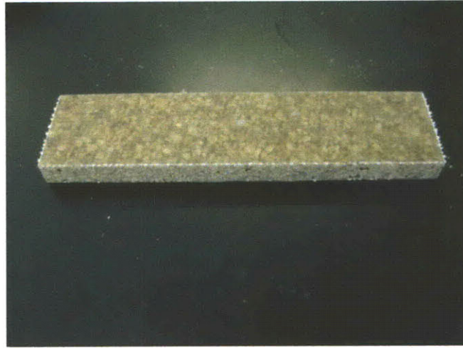
Figure 2.32 A sandwiched cork specimen for bending test
