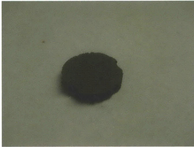
Figure 2.82 A cork specimen after graphite spraying
