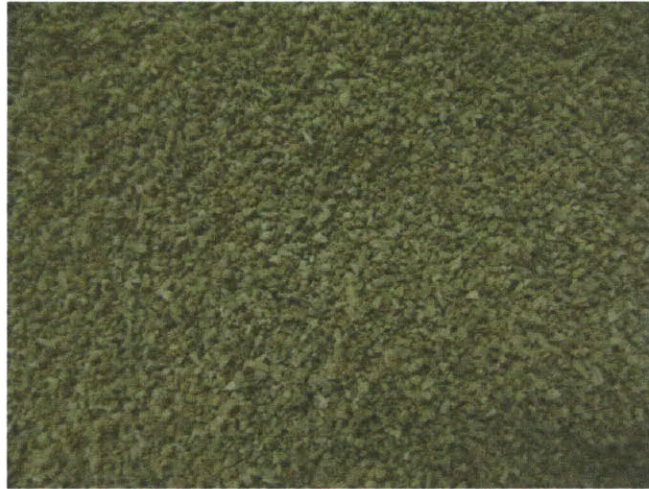
Figure 2.16 The finest cork granules: 1mm
