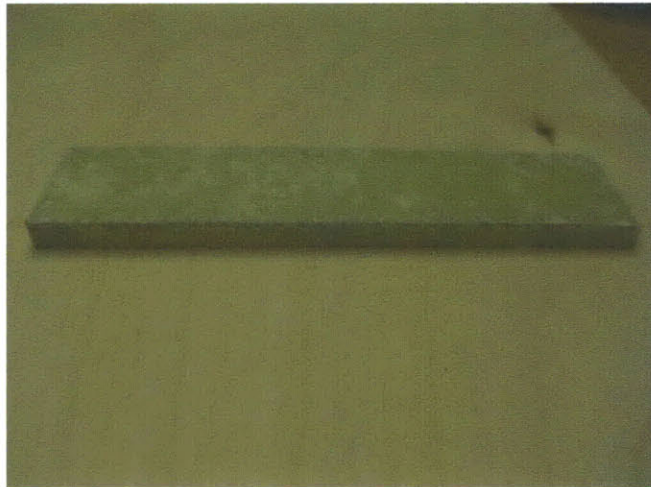
Figure 2.27 A fiberglass specimen for bending test
