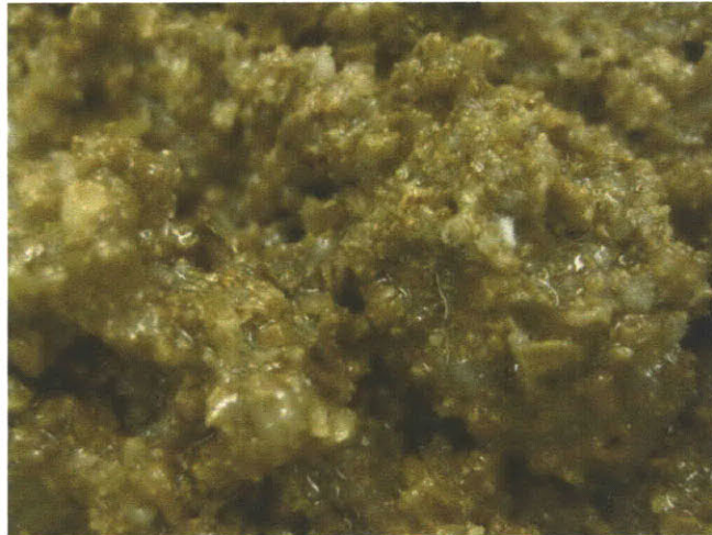
Figure 2.39 Core cork with short fibers and epoxy
