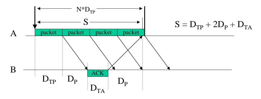
• We want to choose N large enough to allow continuous transmission while waiting for an ACK for the first packet of the window,
