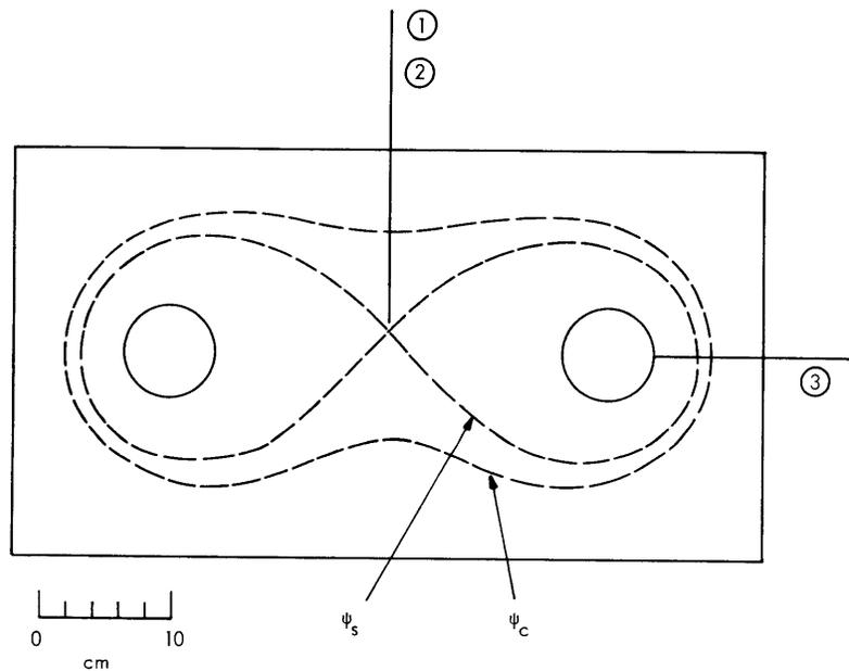
Fig. XIII-7. Cross section of the device showing the locations of the separatrix  $\psi_s$  and critical field line  $\psi_c$ , as well as the paths of the three movable probes.
