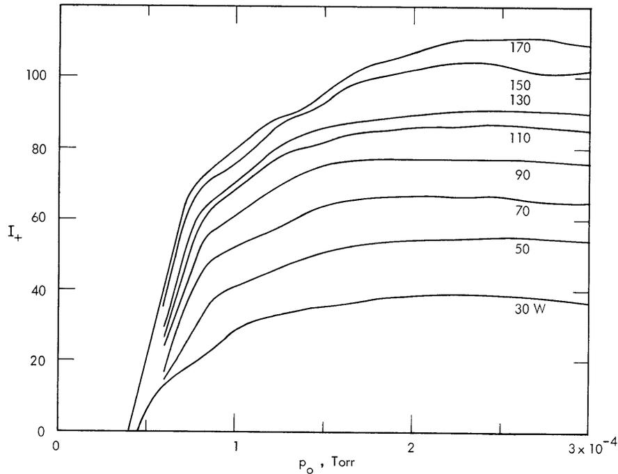
Fig. XIII-10. Ion saturation current vs neutral gas filling pressure with RF power as a parameter.
