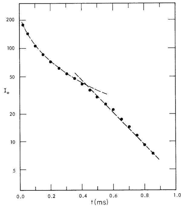
Fig. XIII-9. Decay of ion saturation current with time. RF power off at  $t = 0$ . Points for  $t < 0.4$  ms fitted by  $(1+at)^{-1}$  and for  $t > 0.4$  ms by  $\exp -\beta t$ . ( $a = 10.9 \times 10^3 \text{ s}^{-1}$ ;  $\beta = 3.6 \times 10^3 \text{ s}^{-1}$ .)
