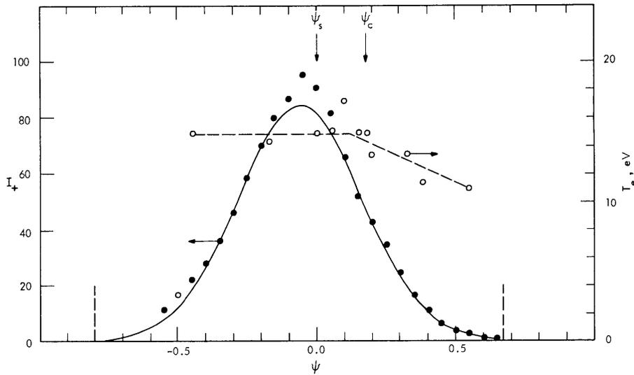
Fig. XIII-8. Scan of ion saturation current and electron temperature measured by Probe 3. Vertical dashed lines show positions of conducting bar and vacuum chamber wall.
