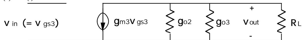
where  $g_{m3} = \sqrt{2K_3I_D} = 10^{-3}$  mS,  $g_{o3} = \frac{I_D}{V_{A3}} = 10^{-4}$  mS,  $g_{o2} = \frac{I_D}{V_{A2}} = 5 \times 10^{-5}$  mS,
