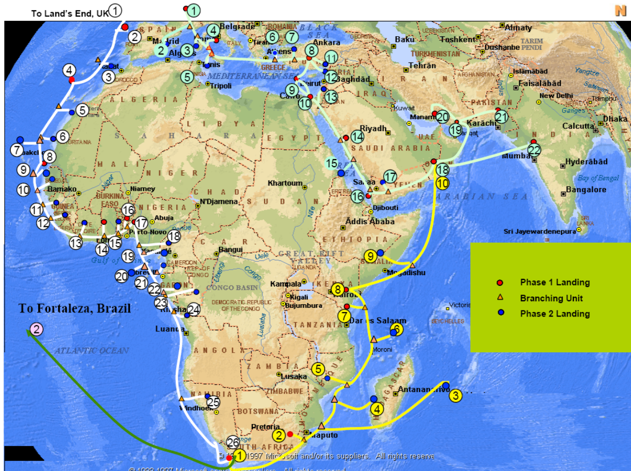
Figure 3.14: Uhurunet Submarine Cable Project Source: NEPAD e-Africa Commission, Accessed 20th July 2009
