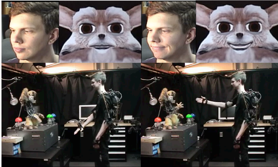
Figure 3-4: Demonstration of motor mimicry. These pictures show two different domains where the motor mapping techniques from this chapter have been demonstrated. The top row shows two human facial expressions and the resulting mimicry performed by the robot. In these examples, the output shown is the result of the process in section 3.3 - once the learning phase is over, the human's facial points are mapped into joint angles, then those joint angles are used as an input to search the robot's pose-graph for the closest animation (or in this case, the closest weighted blend of facial expressions animations). The bottom row shows the robot mimicking the position of the human's arm. In this case, the direct result of the joint mapping 3.2 is being performed.
