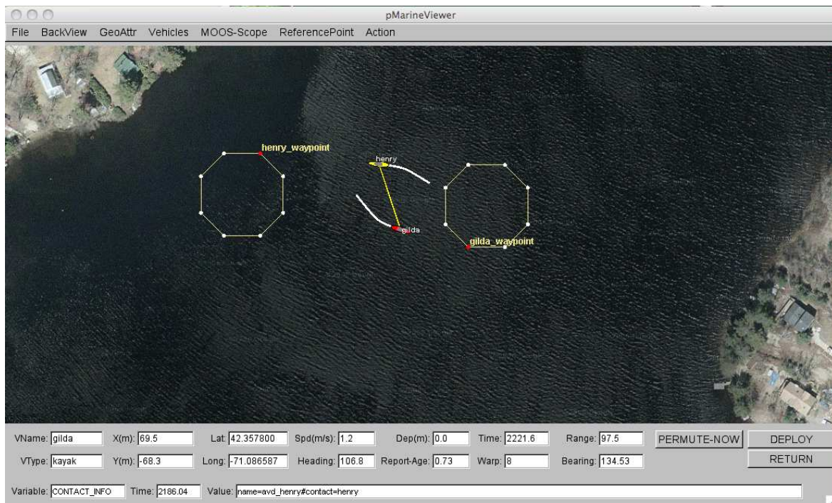
Figure 52: The Berta Mission (2) : The vehicles have changed their loiter stations and this puts them at risk for collision. The green bearing line between the vehicle indicates the presence of the AvoidCollision behavior.
