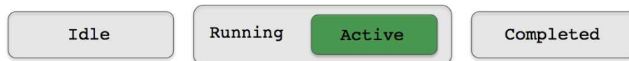
Figure 15: Behavior States: A behavior may be in one of these four states at any given iteration of helm Iterate() loop. The state is determined by examination of MOOS variables stored locally in the helm's information buffer.
