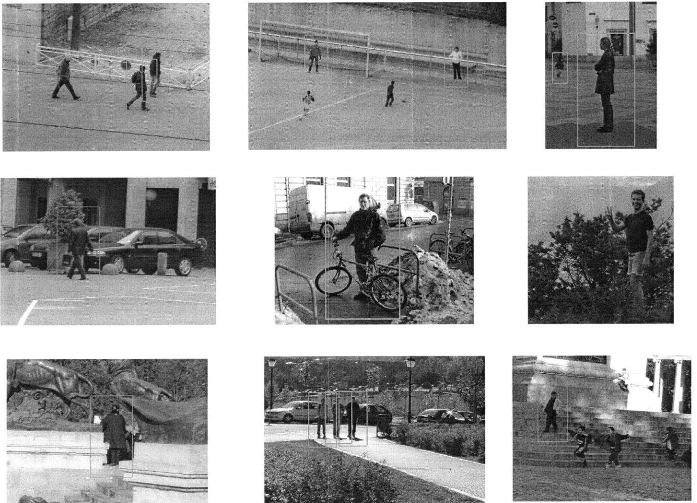
Figure 3-5: Several detection results obtained with our implementation of the Dalal-Triggs algorithm. The downscaling ratio is 1.05 and the window stride is 8 \times 8 .
