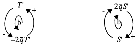
Figure 8a: Feedback loops for mean flow, the ocean’s tendency to reduce variations in temperature and salinity. They represent the right-hand terms in eqs. 51 and 52. Both are balancing and therefore stabilize the equilibria.
