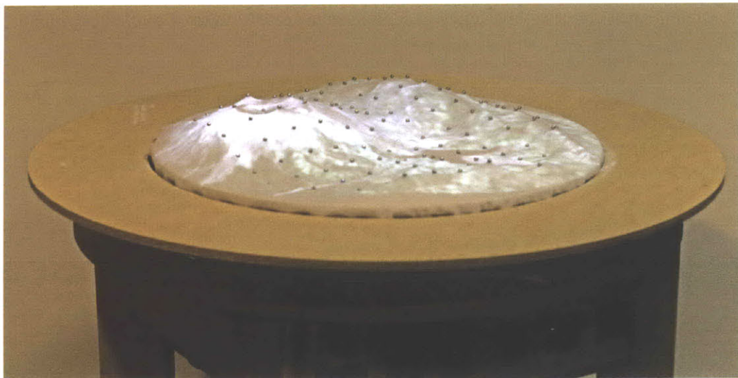
Figure 3-15: Rods covered with spandex fabric and augmented with projected graphics.
