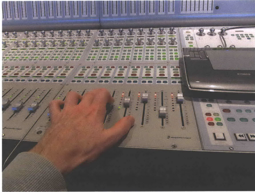
Figure 3-3: Motorized faders on a Digidesign audio mixing console. (Image courtesy of Hens Zimmerman)
