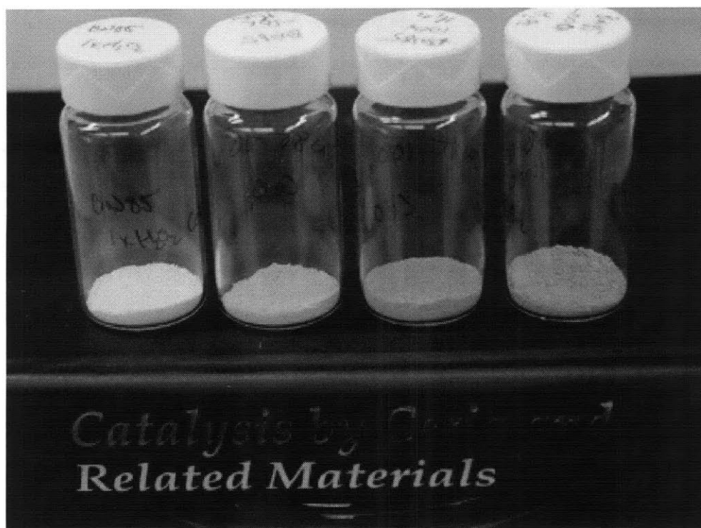
Figure 3-2: As the \text{CeO}_2 nanocrystals dried, they became lighter in color, though still much darker than reported elsewhere. From left to right, 0.058, 0.58, 5.8, and 58:1 \text{H}_2\text{O}_2:\text{CeCl}_3 ratio.
