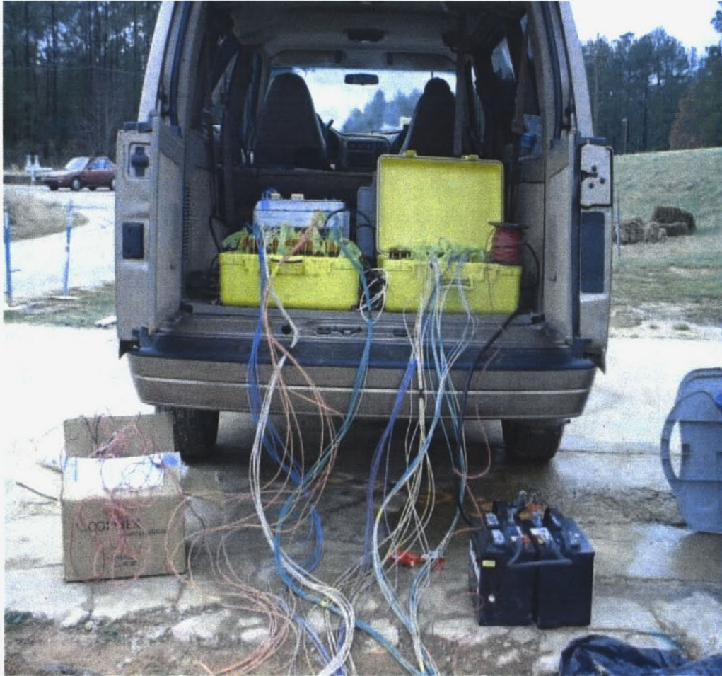
Figure A.2 – Equipment at field site. Yellow boxes are MX-30 multichannel receivers, white box is GDP-32 and gray box is ZT-30 power transmitter.
