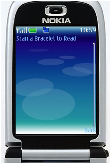
Fig. 4. If the physician selects the option of scanning the NFC tag, he or she is prompted to tap the NFC tag onto the cell phone for reading.
