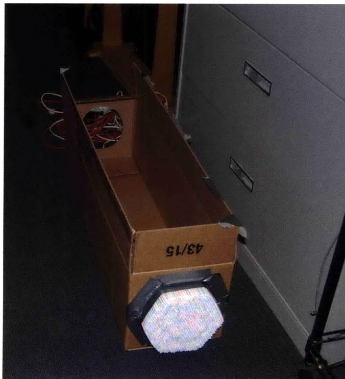
Figure 3.3: Constructed wind tunnel.
