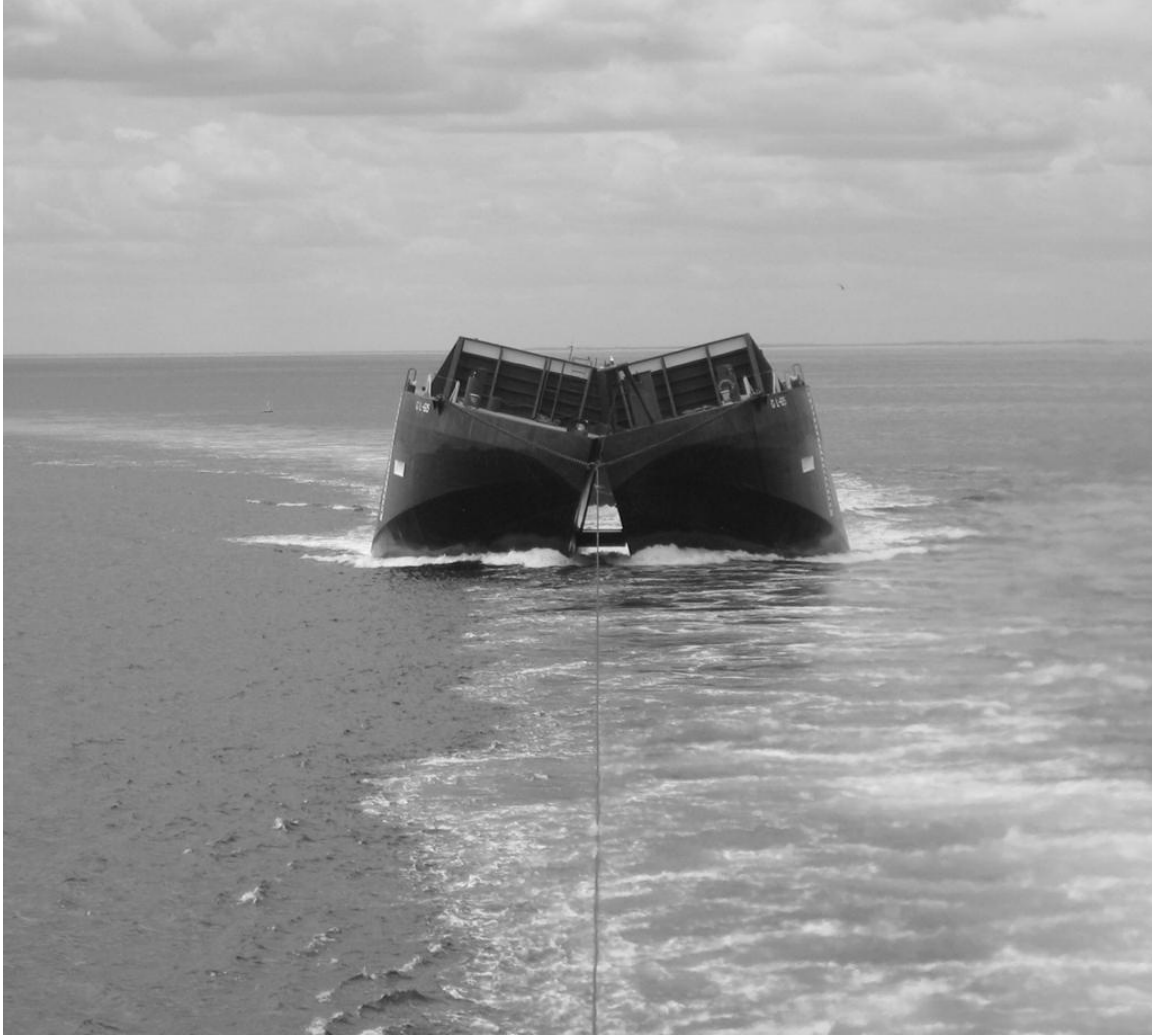
Figure 3-2: Photograph of a split-hull barge, which is an example of a line release ( photo: T. Fredette, 2009 ).
