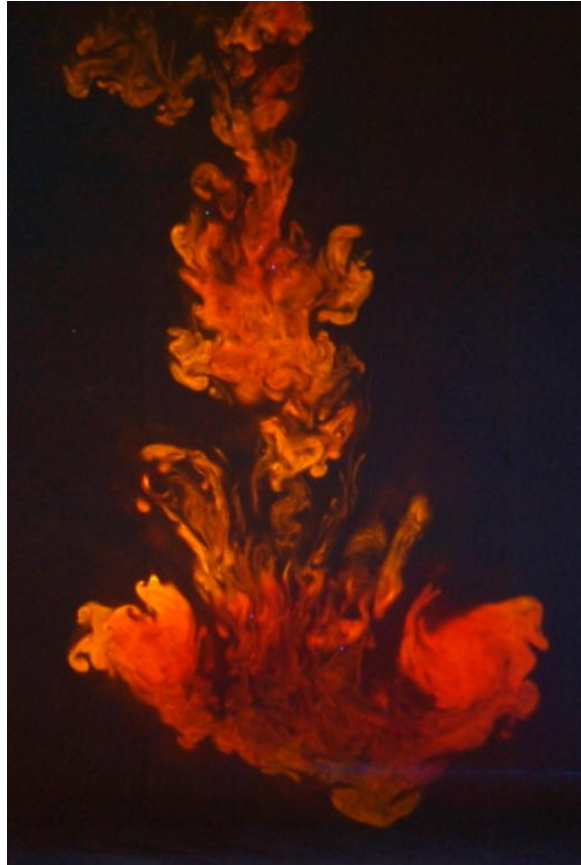
Figure 4-13: The thermal created by dense brine when released from the surface; it has been colored with rhodamine dye to enhance the visualization of the cloud structure. The frame size is approximately 44 cm wide x 55 cm tall.
