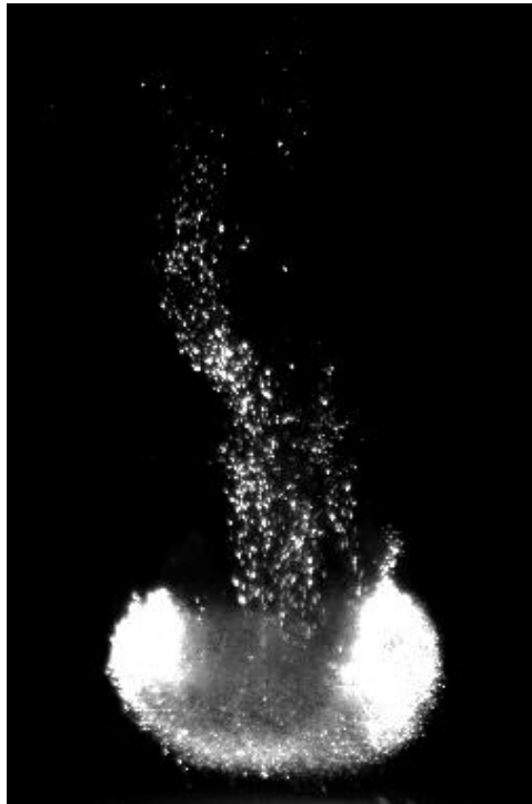
Figure 4-21: An example of a descending particle cloud created with dry, B Glass Beads that were released at the surface in a 6 cm/s ambient current.
