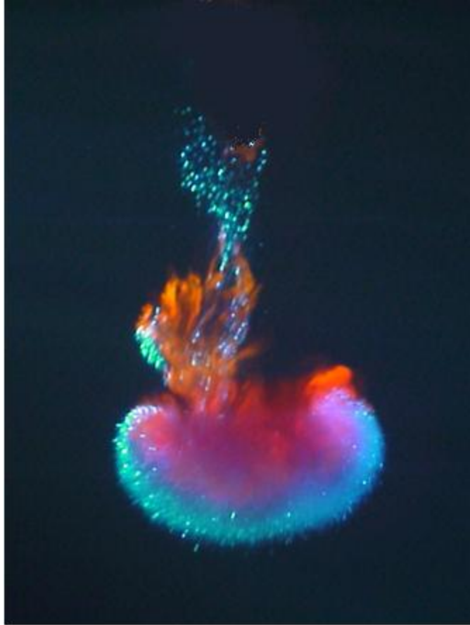
Figure 4-18: The thermal created by B Glass Beads when released from the surface in the saturated condition (with rhodamine dye), into a 6 cm/s current. Note the trailing stem as well as the separation of the fluid and particles. The frame size is approximately 31 cm wide x 55 cm tall.
