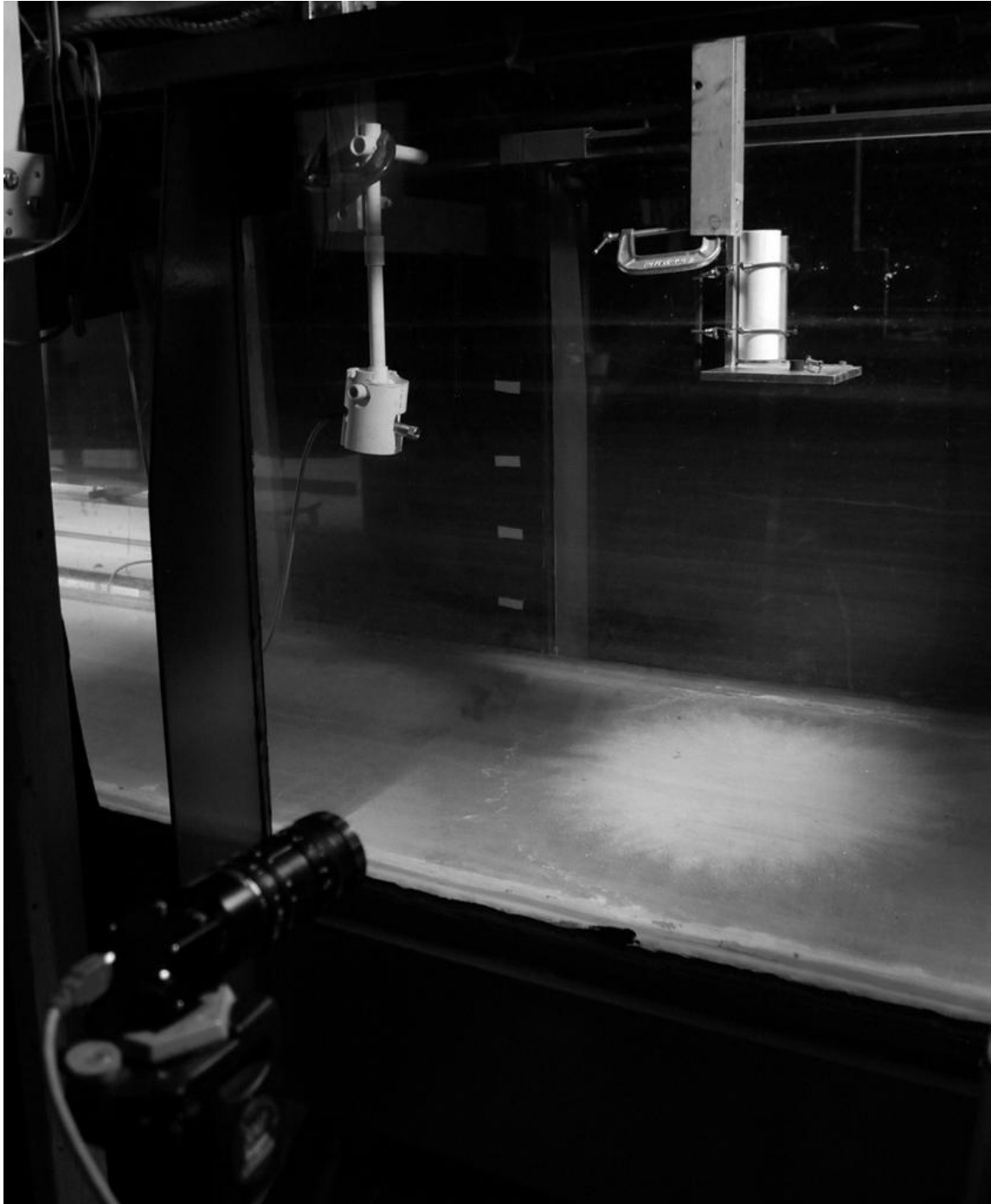
Figure 3-4: The recirculating channel (shown in the drained condition) with the laser head, camera, and release mechanism positioned for experimental trials.
